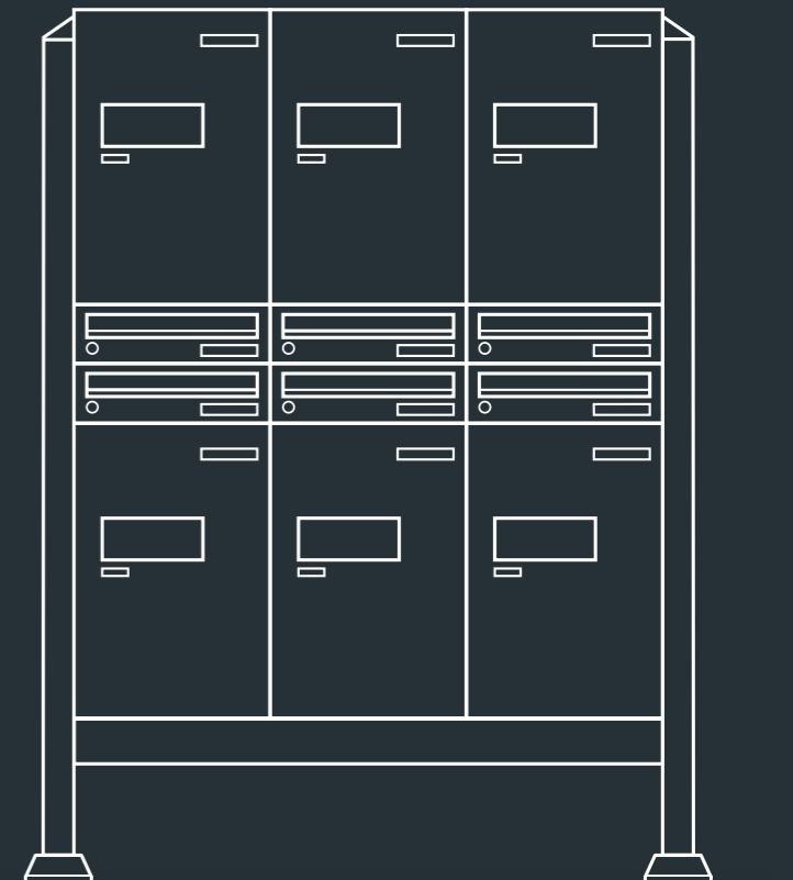
Ideal for use in semi-detached houses and apartment buildings: the eBoxx EASY+ (model E) used as a system combined with the eBoxx letterbox A, Terzo post and Terzo foot.
