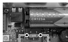
Fig. 5: Slide switch for selecting the power supply supply
