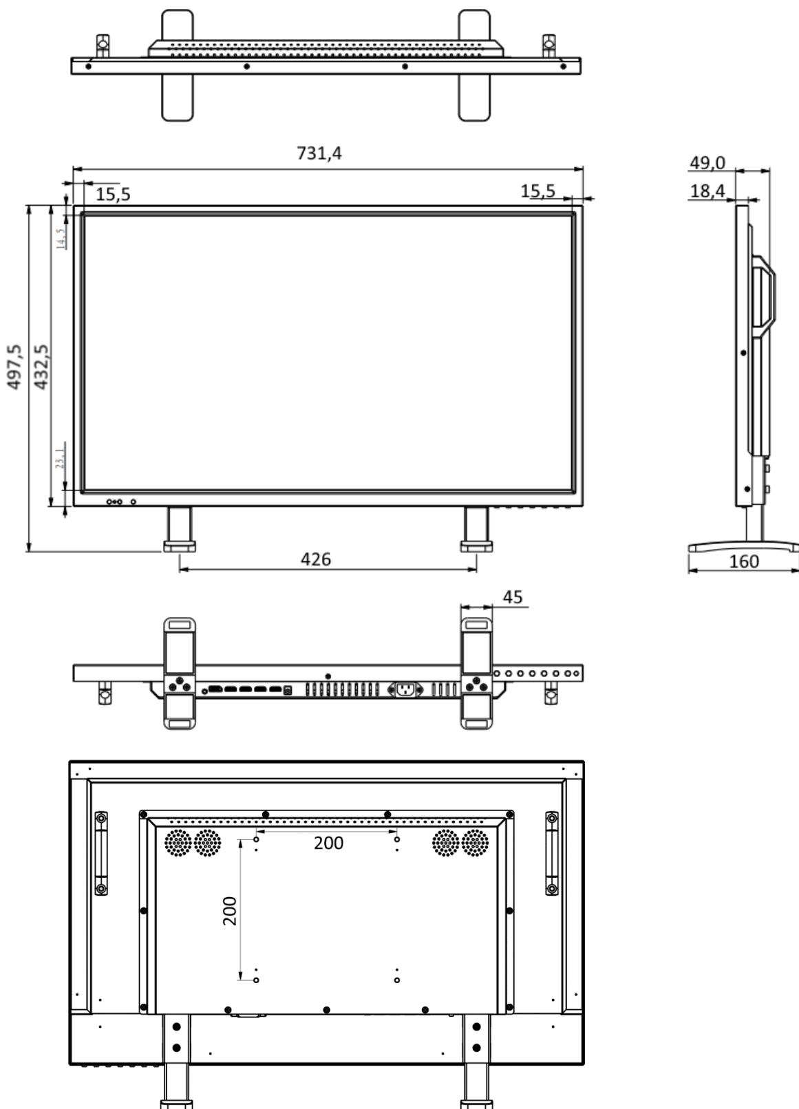
All dimensions in millimeter. Drawings not true to scale.
