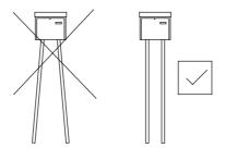
b. In all the directions, the stand shall be at a 90° angle to the ground.
