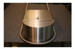
5. Open the door (if necessary, an assisting person can secure it against closing). Insert the screws through the holes from inside and use the black half-round spacers to screw them onto the stand (without tightening them completely). Always begin with the holes positioned nearer to the box top panel.
