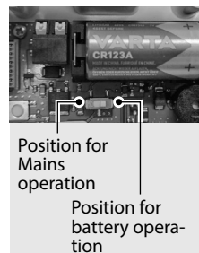
Fig. 5: Slide switch for selecting the power supply supply
