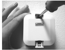
Fig. 19: Loosening the extender
