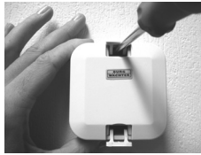
Fig. 14: Mounting the extender
