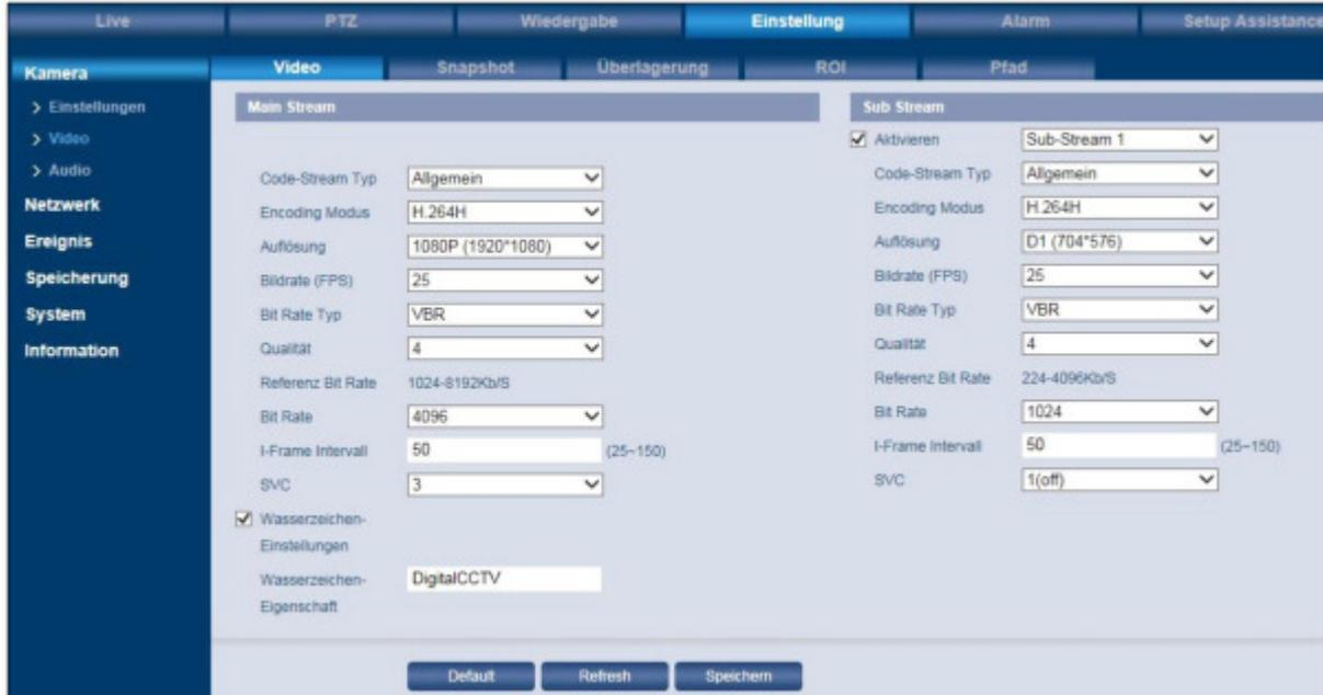
The screenshot shows the 'Einstellung' (Settings) tab for a camera, specifically the 'Video' sub-tab. It is divided into two main sections: 'Main Stream' and 'Sub Stream'.
