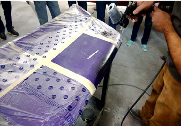
Spray Base Coat
