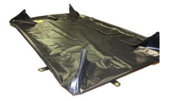
Slide L-brackets into the Berm pockets to support the sidewalls. Do this for all but the one wall that will be used to load the spill pallet and IBC. (NOTE: the longer (17") side of the bracket should be inserted into the sleeve. The shorter (11") side will go underneath the berm.)
