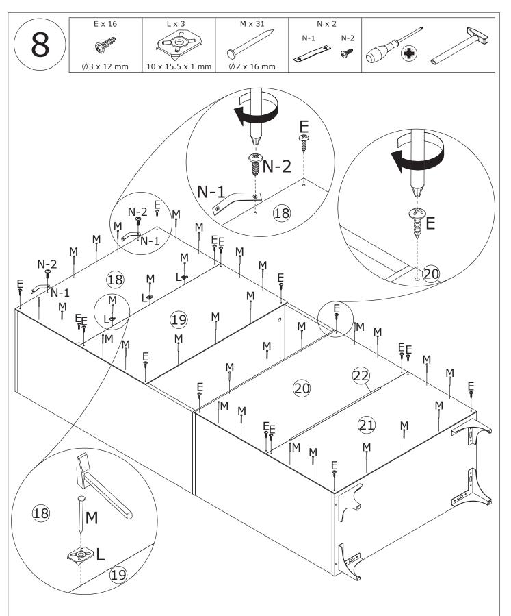
Connect board 20 and 21 to strip 22 at first. Fix back board 18, 19, 20 and 21 to the cabinet with nail(M) and screw(E) as shown. Use iron sheet(L) to fix board 18 and 19 with nail(M) as shown. Fix strip(N-1) to board 18 with screw(N-2).
