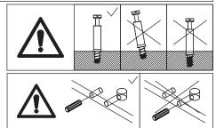
Attach board 1 and 9 to board 2 and 3 using wooden dowel(C), and fix with screw(D) as shown.
