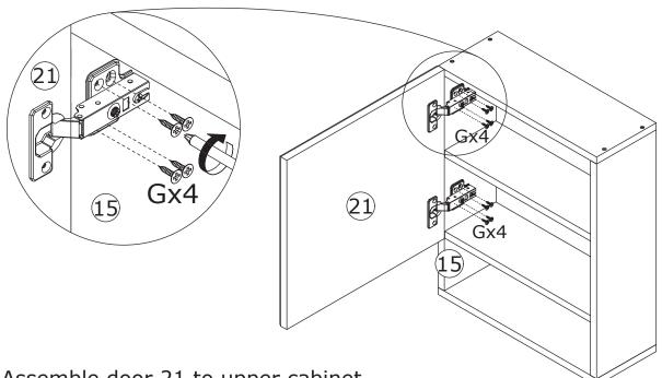
Assemble door 21 to upper cabinet by fixing hinge with screw(G) as shown.
