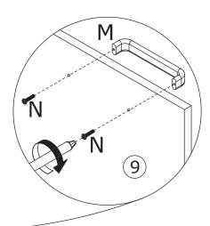
Fix handle(M) to board 9 with screw(N) as shown.
