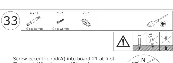
Fix handle(N) with screw(C) as shown.
