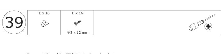
Insert buckle(E) into back slots and fix with screw(H) as shown.
