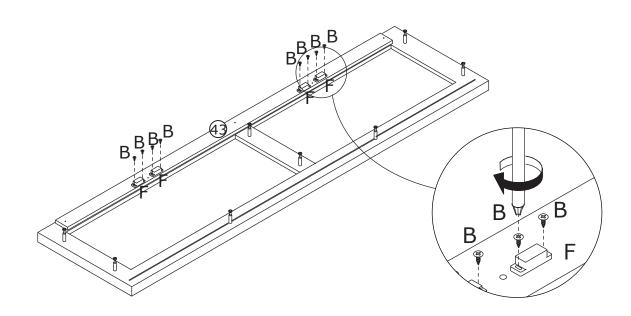
Fix part(F) to board 43 with screw(B) as shown.
