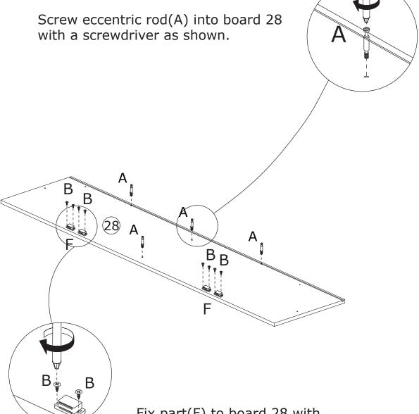
Fix part(F) to board 28 with screw(B) as shown.
