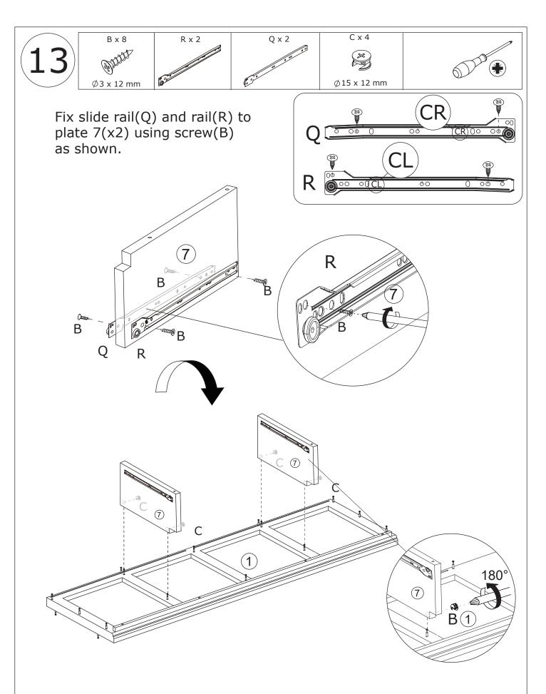
Attach plate 7 to plate 1,insert cam lock(C) into holes in plate 7 and turn clockwise to tighten as shown.
