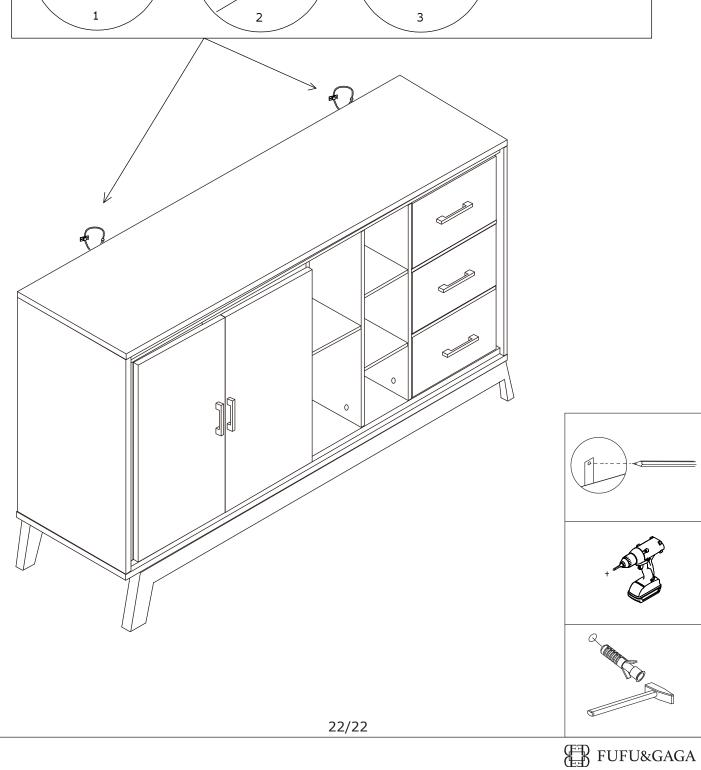
If there is misalignment after you install, adjust the screw to the best condition
