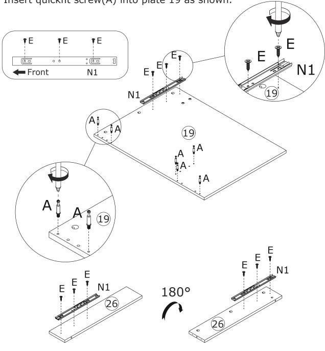
Fix slide rail(N1) to two sides of plate 26 with screw(E) as shown.
