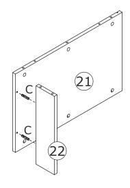
Attach plate 22 to plate 21 with wooden dowel(C) as shown.
