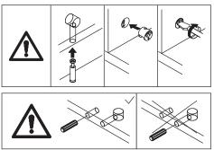
Connect the two assembled components using wooden dowel(G), add cam lock(H) into and turn clockwise to tighten as shown.
