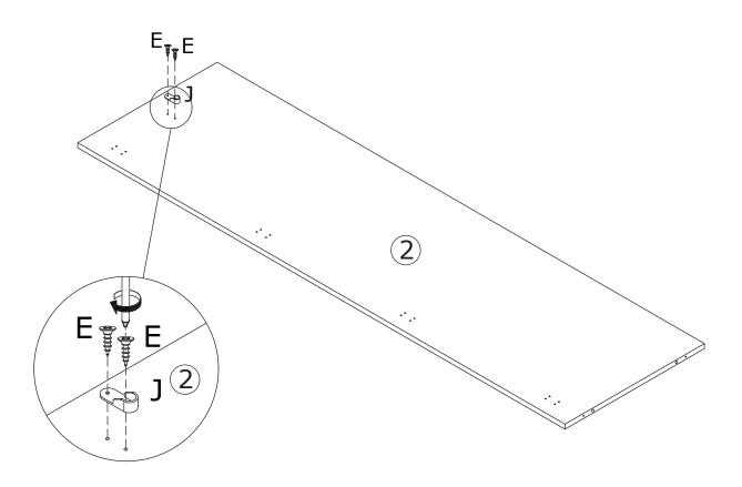
Fix part(J) to board 2 and 4 with screw(E) as shown.
