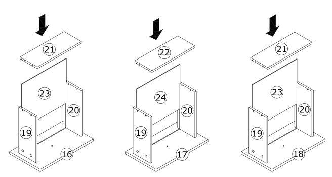
Insert bottom board 23 and 24 along available grooves as shown.
