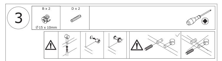
Attach plate 3 to plate 5 with wooden dowel(D) and turn cam locks(B) clockwise to tighten as shown.
