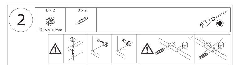
Attach plate 5 to plate2 with wooden dowel(D) and turn cam locks(B) clockwise to tighten as shown.
