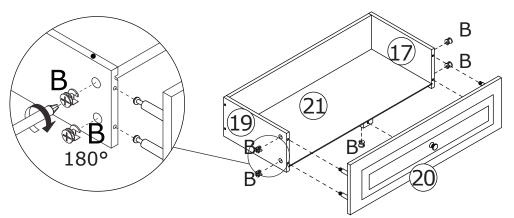
Attach plate 25 to the component and turn cam locks(B) clockwise to tighten as shown. Please pay attention to the holes where the accessories are inserted. Fix runner(DL) and (DR) to plate 19 and 17 respectively
