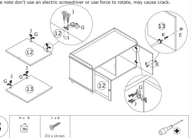
Use part H to fix back panel using bolts J as shown.
