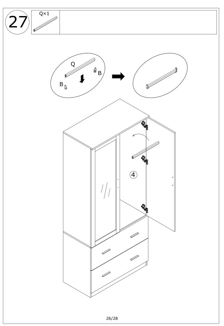
Adjust the length of hinges to avoid a gap between doors.
