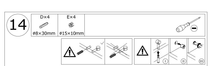
Connect 2 assembled components using wooden dowel D and lock with cam locks E as shown.
