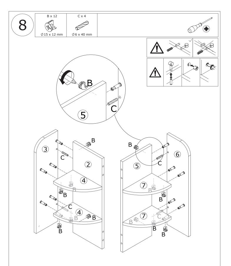
Knock wooden dowel(C) slightly into side of No.2 and No.5 plate respectively at first. Attach No.3 plate to No.2 and No.4; No.6 plate to No.5 and No.7, then turn cam lock(B) in No.2,4,5,7 plates clockwise to tighten as shown.
