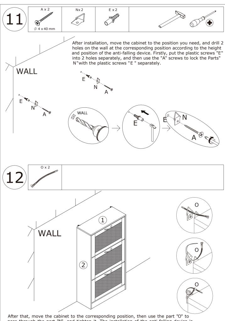
After that, move the cabinet to the corresponding position, then use the part "O" to pass through the part "N", and tighten it. The installation of the anti-falling device is completed.
