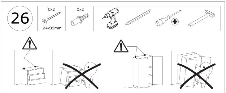
Install anti-tipping device as shown.
