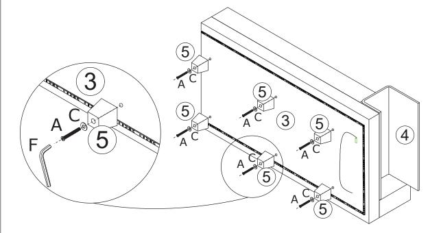
Fix leg #5 to part #3 using washer(C) and screw(A) as shown.
