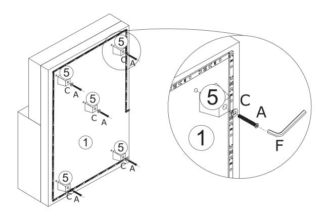
Fix leg #5 to part #1 using washer(C) and screw(A) as shown.
