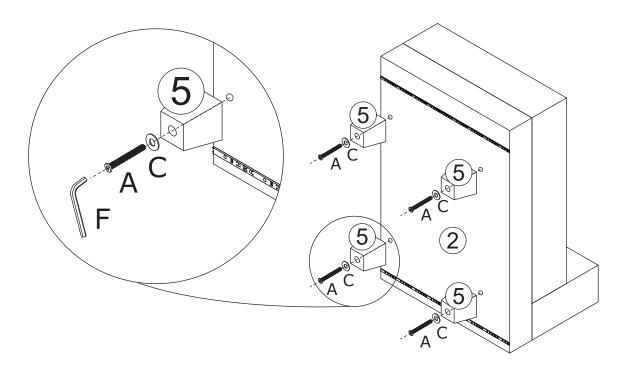
Fix leg #5 to part #2 using washer(C) and screw(A) as shown.
