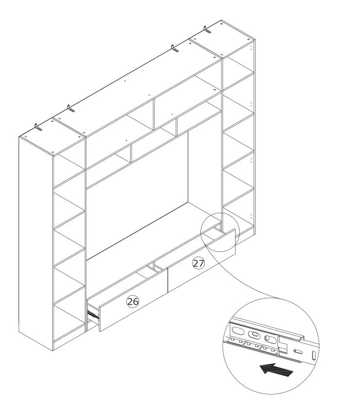
Align rails, insert drawers into corresponding position.
