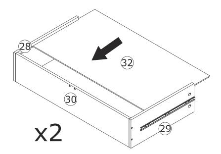
Insert bottom board 32 along available grooves as shown.
