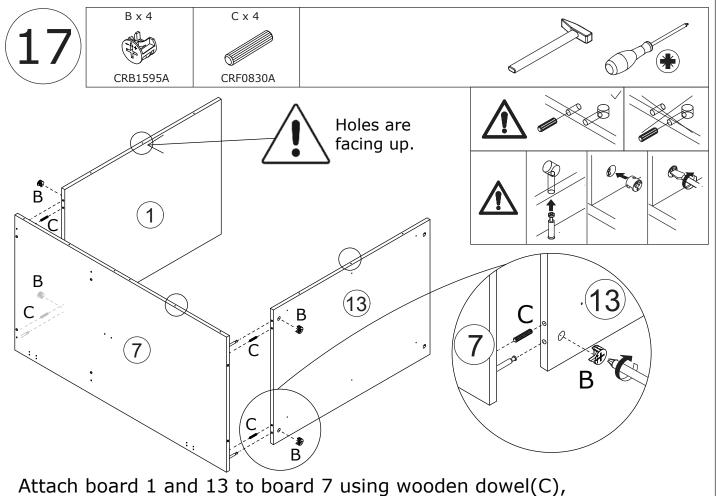
add cam lock(B) into and turn clockwise to tighten as shown.
