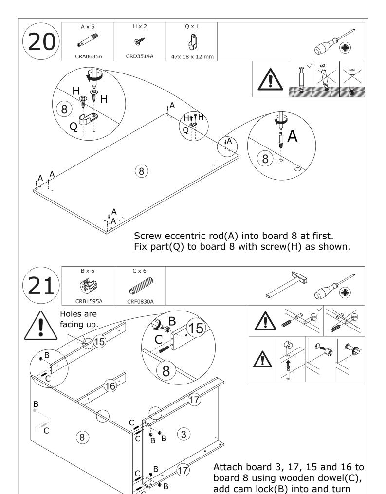
clockwise to tighten as shown.
