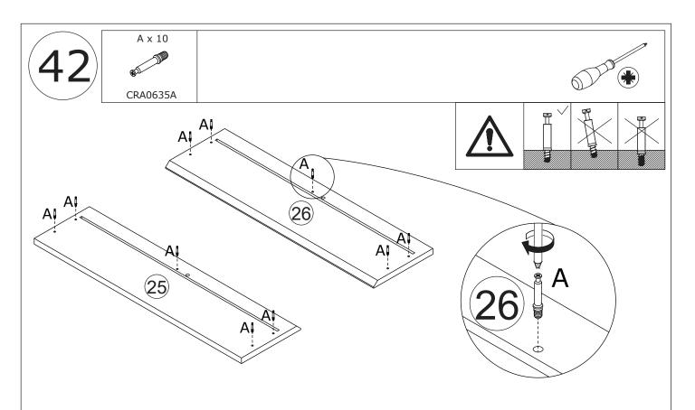
Screw eccentric rod(A) into board 25 and 26 at first.
