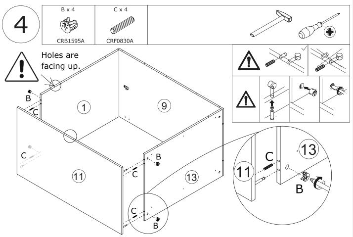
Connect board 11 to board 1 and 13 to using wooden dowel(C), add cam lock(B) into board 1,13 and turn clockwise to tighten as shown.  $$^{8/40}$$
