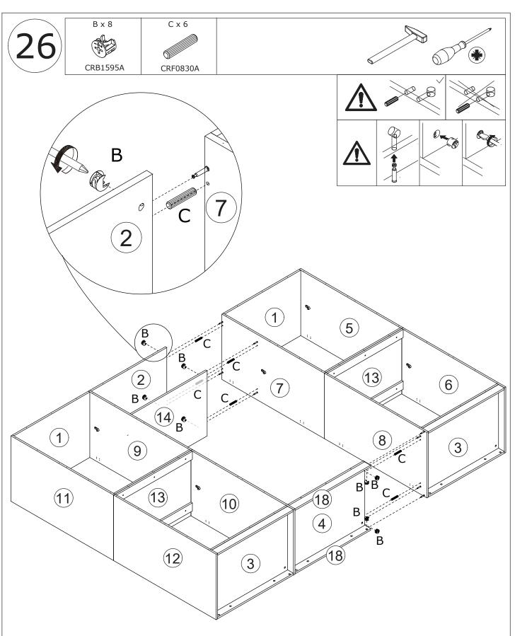
Attach the component (assembled in step 15) to board 7 and 8 using wooden dowel(C), add cam lock(B) into and turn clockwise to tighten as shown.
