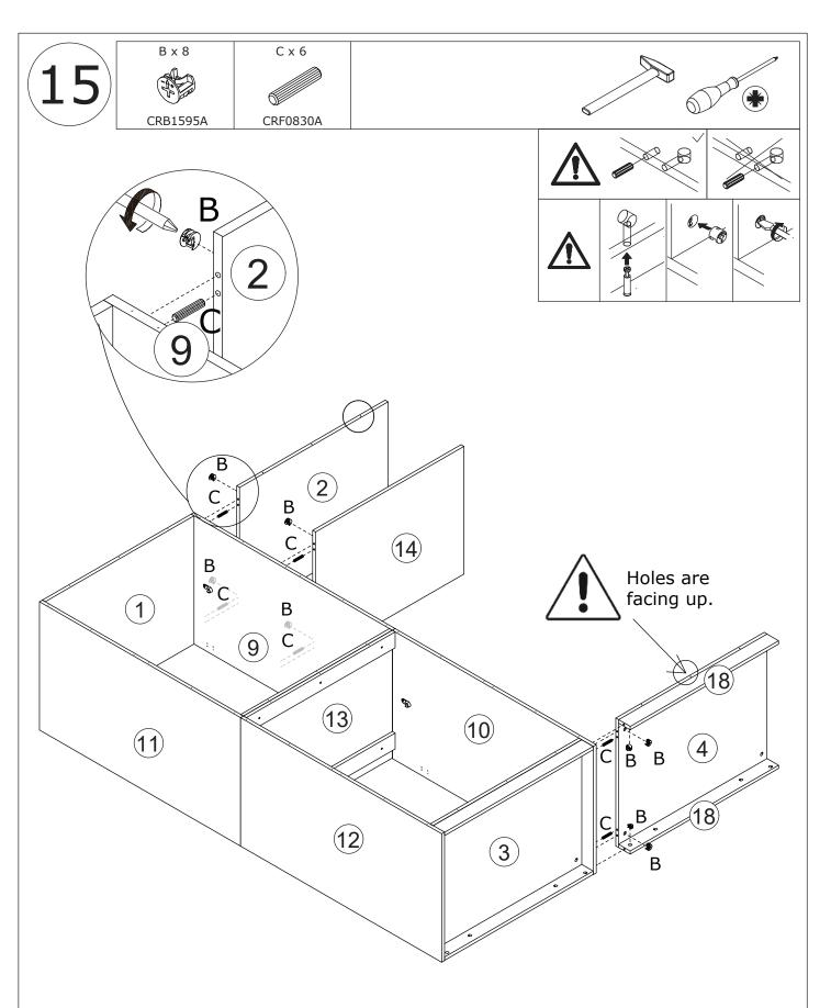
Attach board 4, 14 and 2 to board 10 and 9 using wooden dowel(C), add cam lock(B) into and turn clockwise to tighten as shown.
