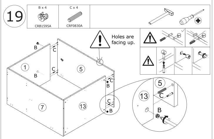
Attach board 5 to board 1 and 13 using wooden dowel(C), add cam lock(B) into and turn clockwise to tighten as shown.
