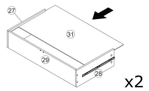
Insert bottom board 31 along grooves as shown.
