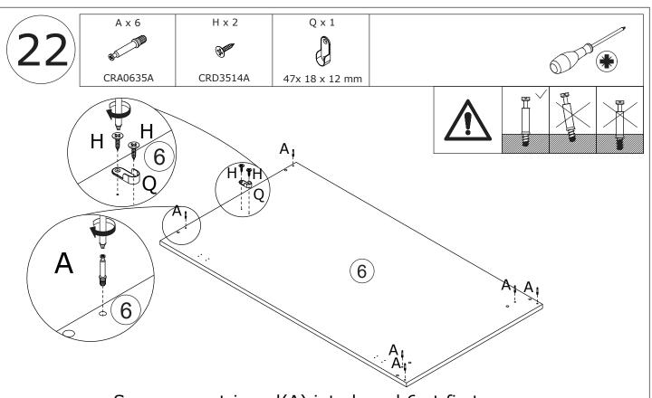
Screw eccentric rod(A) into board 6 at first. Fix part(Q) to board 6 with screw(H) as shown.
