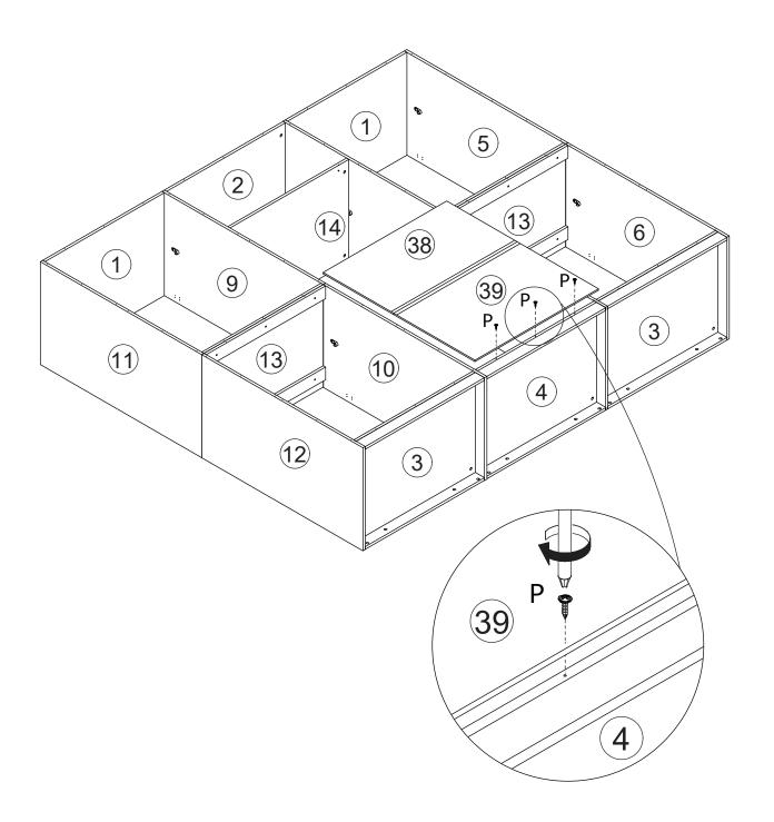
Fix back board 38 and 39 to board 4 with screw(P) as shown.
