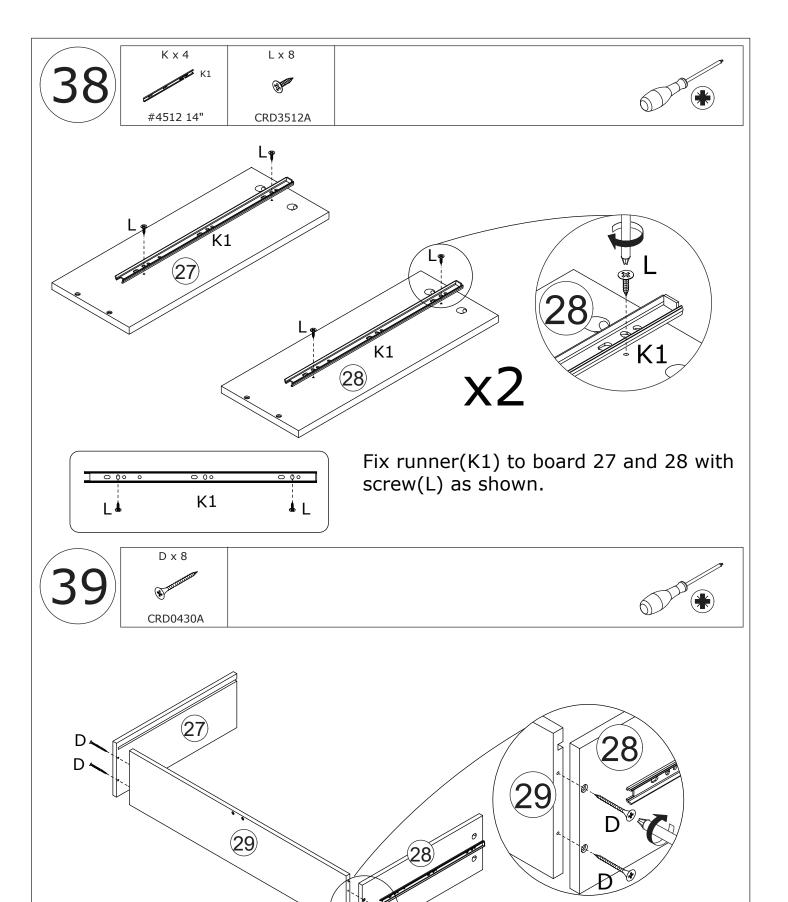
Fix board 27 and 28 to board 29 with screw(D) as shown.
