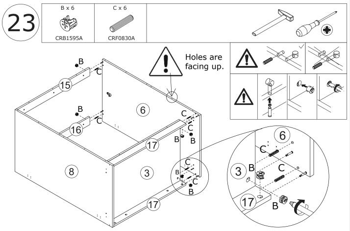
Attach board 6 to board 3, 17, 15 and 16 using wooden dowel(C), add cam lock(B) into and turn clockwise to tighten as shown.
