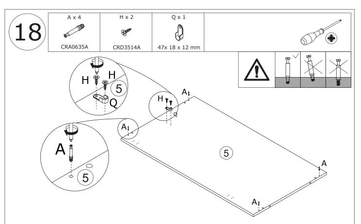
Screw eccentric rod(A) into board 5 at first. Fix part(Q) to board 5 with screw(H) as shown.
