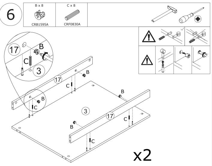
Attach board 17 to board 3 using wooden dowel(C), add cam lock(B) into board 17 and turn clockwise to tighten as shown.
