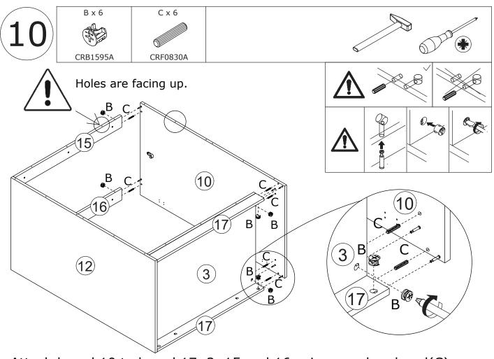
Attach board 10 to board 17, 3, 15 and 16 using wooden dowel(C), add cam lock(B) into and turn clockwise to tighten as shown.
