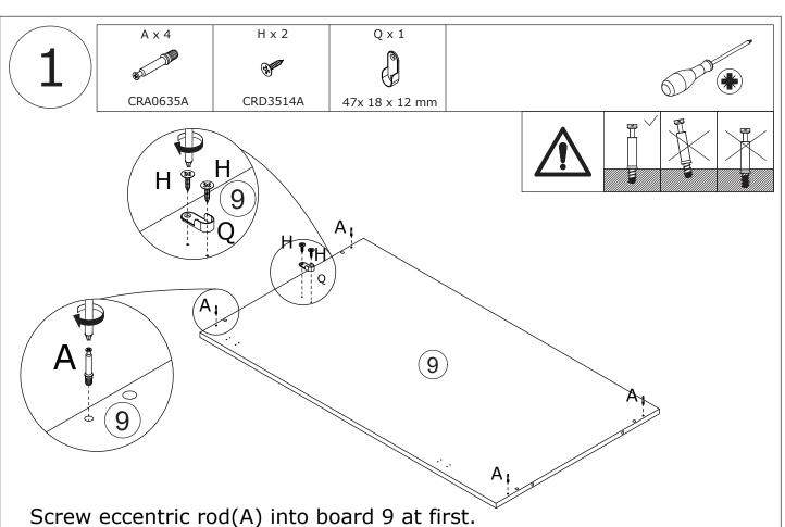
Screw eccentric rod(A) into board 9 at first. Fix part(Q) to board 9 with screw(H) as shown.
