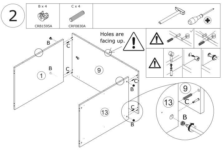
Connect board 1 and 13 to board 9 using wooden dowel(C), add cam lock(B) into board 1,13 and turn clockwise to tighten as shown.
