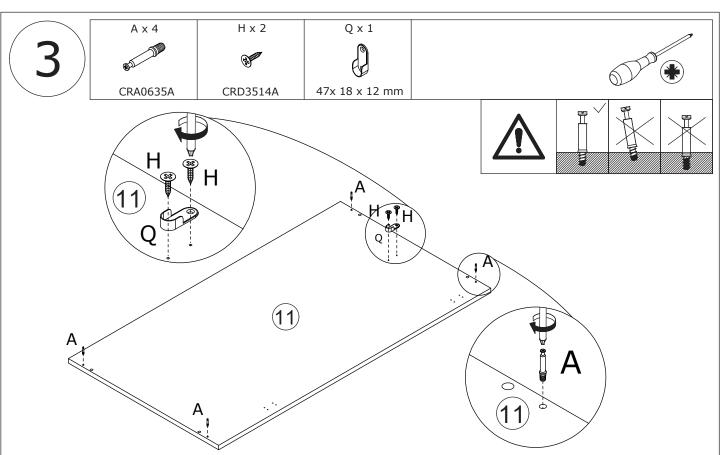
Screw eccentric rod(A) into board 11 at first. Fix part(Q) to board 11 with screw(H) as shown.
