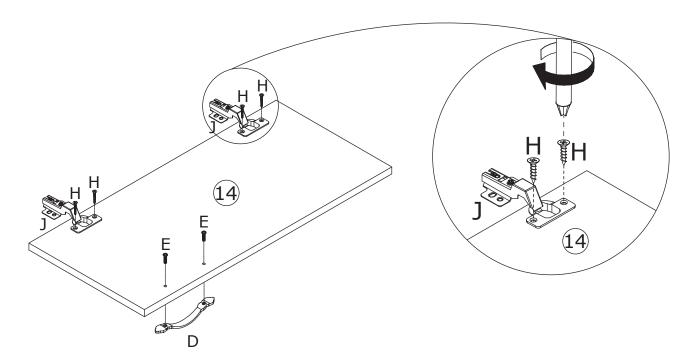
Fix hinge(J) to board 14 and 15 with screw(H) as shown. Fix handle(D) with screw(E) as shown.
