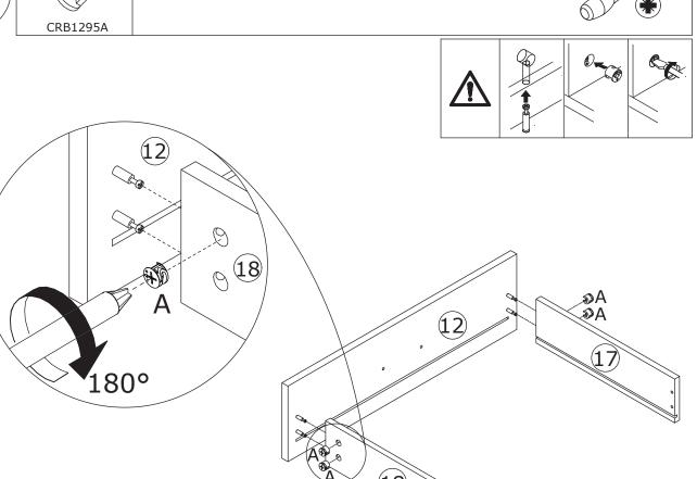
Attach board 12/13 to boarrd 17 and 18, add cam lock(A) and turn clockwise to tighten as shown.
