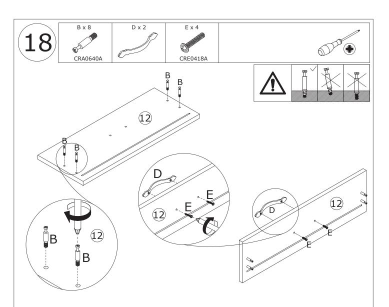
Screw eccentric rod(B) into board 12 and 13 at first. Fix handle(D) with screw(E) as shown.
