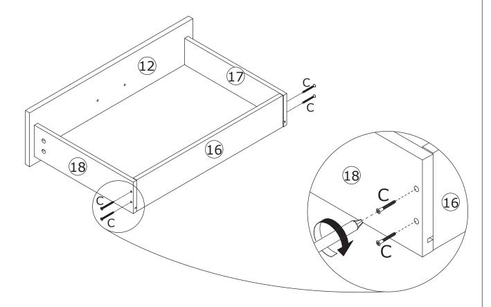
Fix board 16 to board 17 and 18 with screw(C) as shown.
