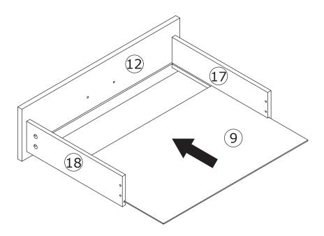
Insert bottom board 9 along grooves as shown.
