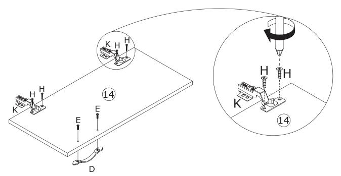
Fix hinge(K) to ANOTHER board 14 and 15 with screw(H) as shown. Fix handle(D) with screw(E) as shown.
