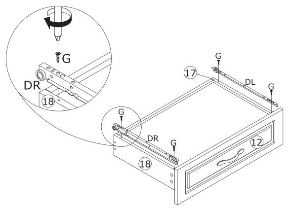
Fix runner(DL) and (DR) to board 17 and 18 respectively with screw(G) as shown.
