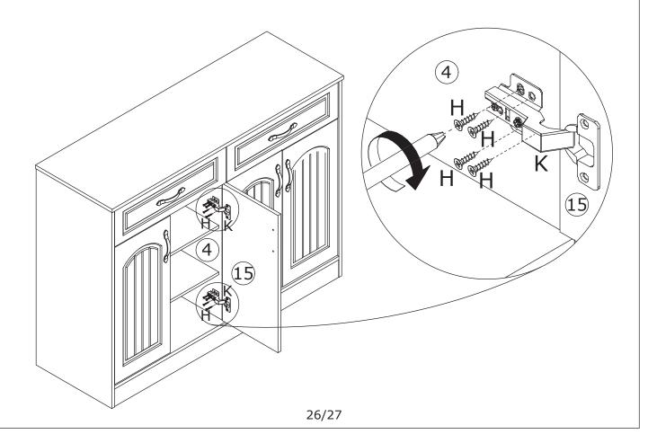
If doors are still not aligned if the hinges are properly correctly, please watch the video.
