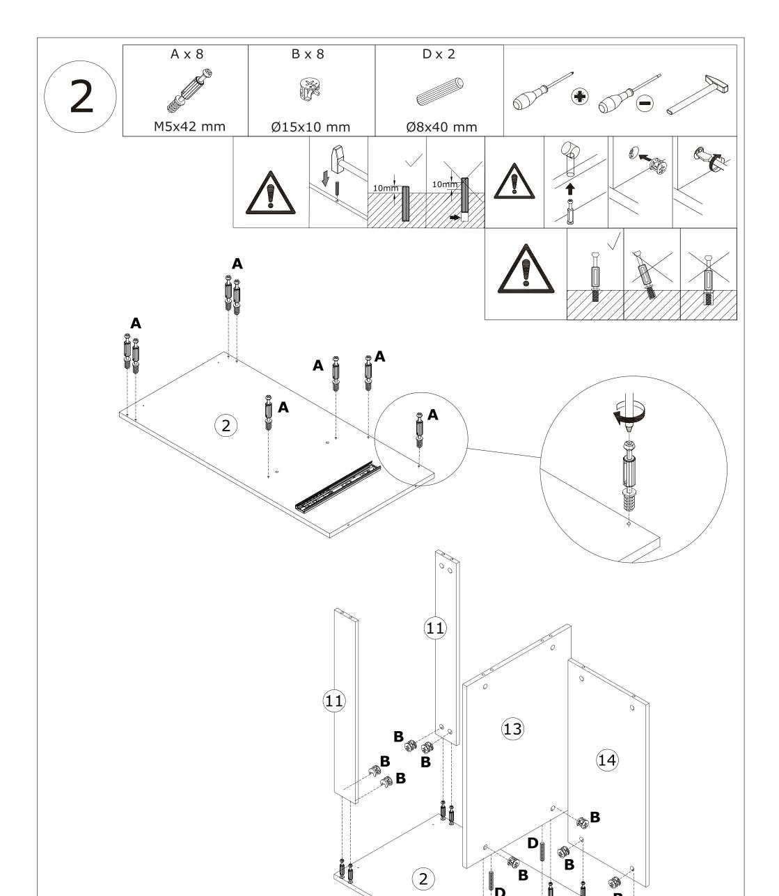
Insert quickfit screw(A) into corresponding holes in plate 2 with a screwdriver as shown. Insert wooden dowel(D) into plate 13 at first. Attach plate 11(x2), 13 and 14 to plate 2, put cam lock(B) into holes in plate 11,13,14 and turn clockwise to tighten as shown.  $_{7/30}$
