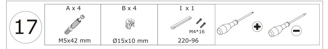
Insert quickfit screw(A) into plate 17 with a screwdriver as shown. Fix handle(I) to plate 17.
