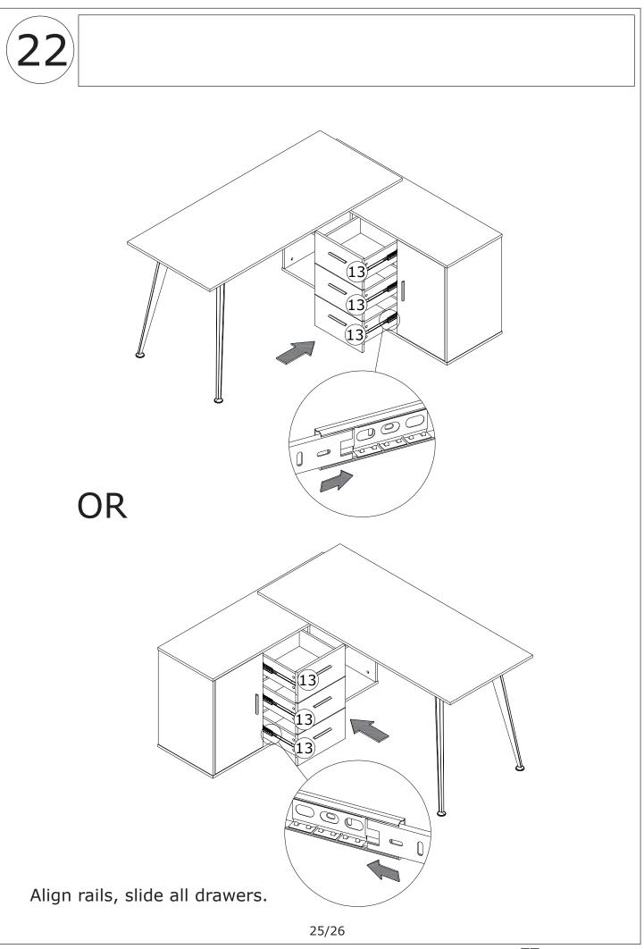
If there is misalignment after you install, adjust the screw to the best condition
