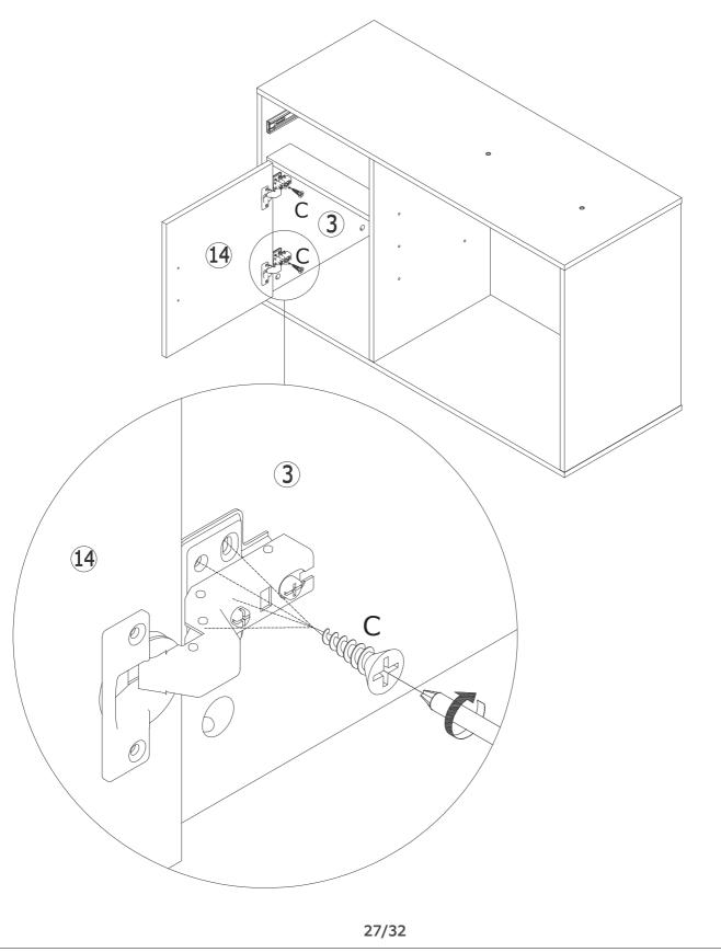
If there is misalignment after you install, adjust the screw to the best condition
