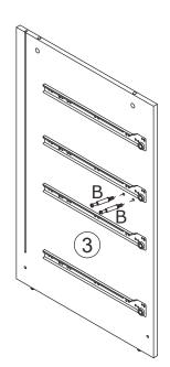
Insert quickfit screw(B) into corresponding holes in board 2,3,4 with a screwdriver as shown.
