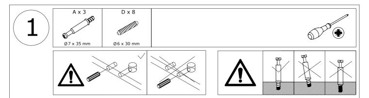
Cam Bolt (A) to plates 2 and 3 with a cross screwdriver, as shown.
