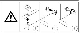
Please cover No. 8 plate on No.2,3, and 4 plates and lock them with Cam Lock(B),as shown.
