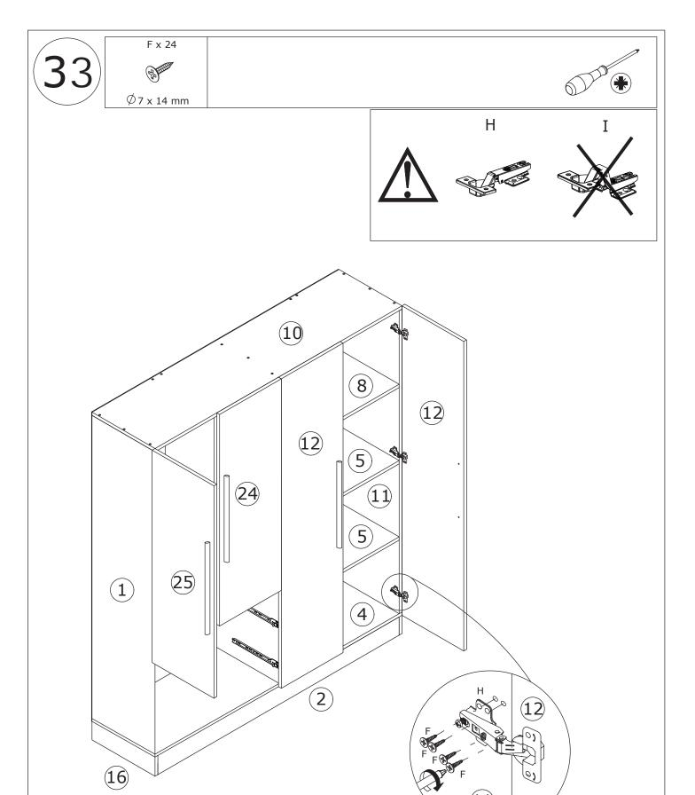
Attach board 25 to board 1, attach another board 12 to board 11 by fixing hinge(H) with screw(F) as shown.
