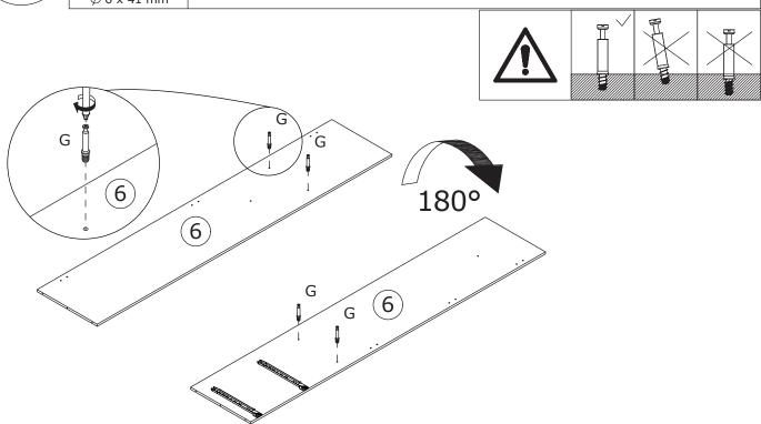
Insert quickfit screw(G) into corresponding holes in board 6 at first.
