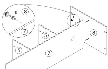
Attach board 8 to board 7, put cam lock(E) into holes in board 7 and turn clockwise to tighten as shown.
