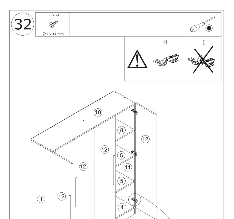
Attach another two board 12 to board 1 and 11 by fixing hinge(H) with screw(F) as shown.
