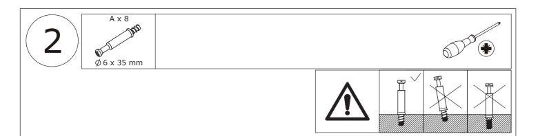
Insert quickfit screw(A) into No.3 and **both sides** of No.4 plate with a screwdriver as shown.
