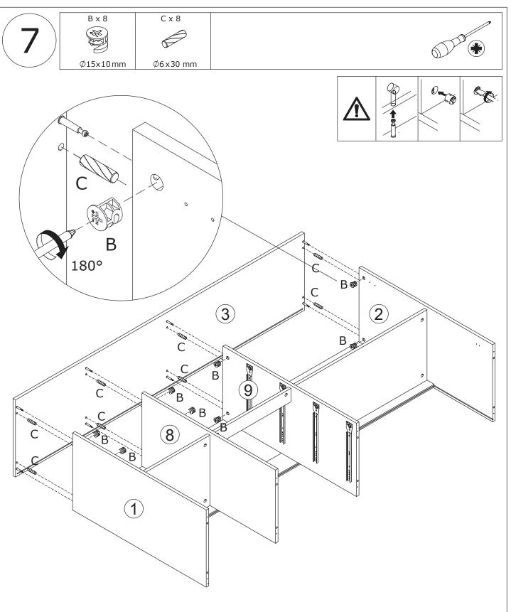
Attach board 3 to the component using wooden dowel(C), add cam lock(B) into board 1,8,9,2 and turn clockwise to tighten as shown.
