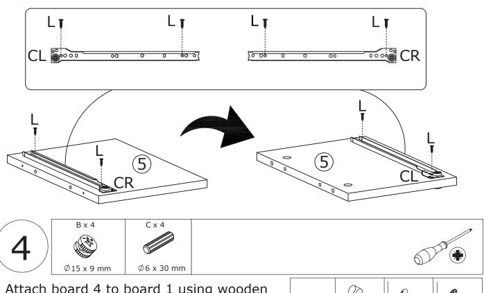
Attach board 4 to board 1 using wooden dowel(C), add cam lock(B) into board 4 and turn clockwise to tighten as shown.
