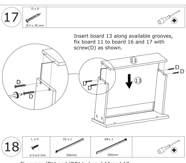
Fix runner(DL) and (DR) to board 16 and 17 respectively with screw(L) as shown.
