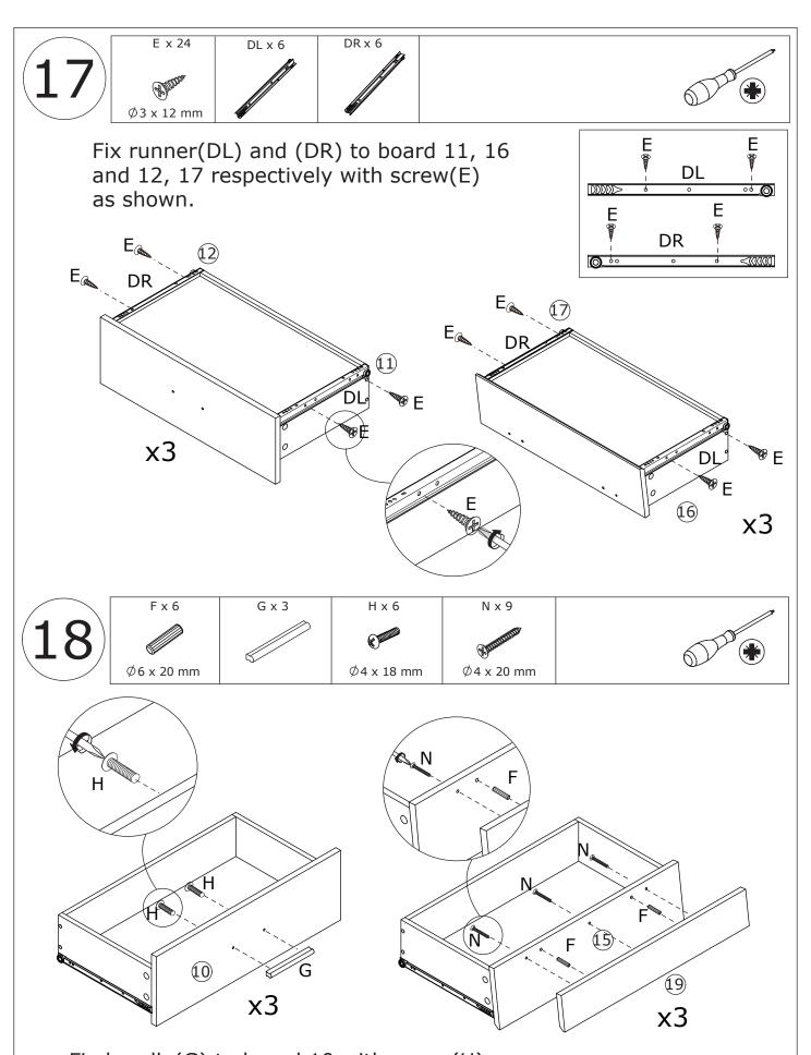
Fix handle(G) to board 10 with screw(H). Attach board 19 to board 15 using wooden dowel(F), then fix with screw(N) as shown.
