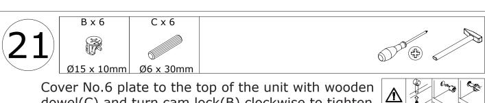
dowel(C) and turn cam lock(B) clockwise to tighten as shown.
