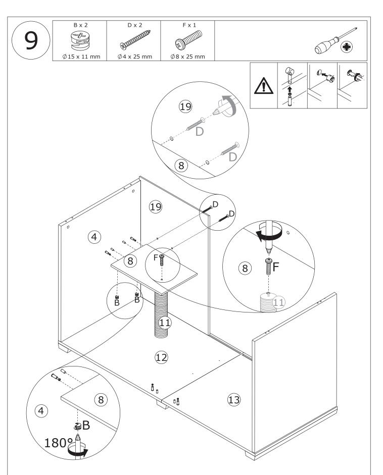
Attach board 8 to board 4, add cam lock(B) into and turn clockwise to tighten as shown. Fix board 8 to part 11 with screw(F), to board 19 with screw(D) as shown.
