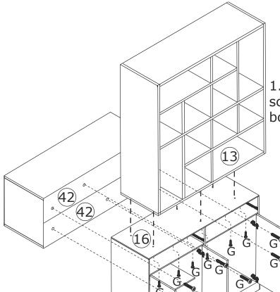
1.Fix board 42 to board 28 with screw(G) and fix board 13 to board 16 with screw(G) as shown.
