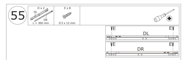
Fix runner(DL) and (DR) to board 33 and 34 with screw(E) as shown.
