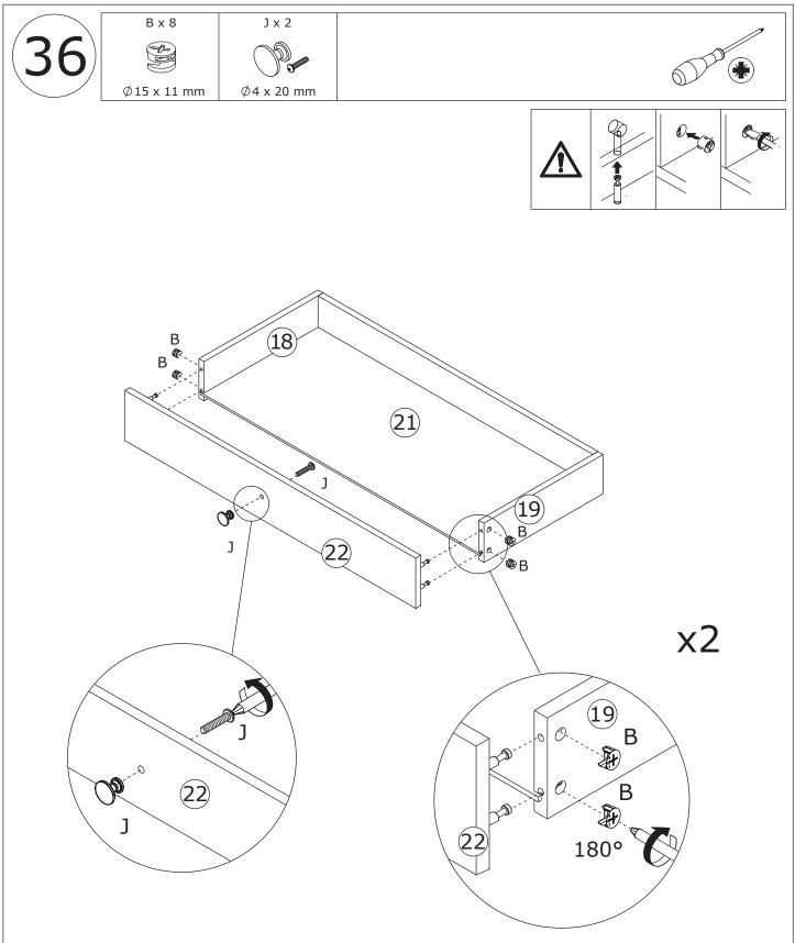
Connect board 22 to board 18 and 19, add cam lock(B) into and turn clockwise to tighten as shown. Fix knob(J) to board 22 as shown.
