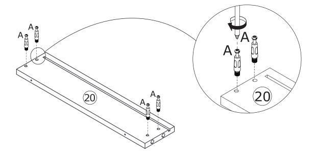
Insert quickfit screw(A) into plate 20 and 23 with a screwdriver as shown.
