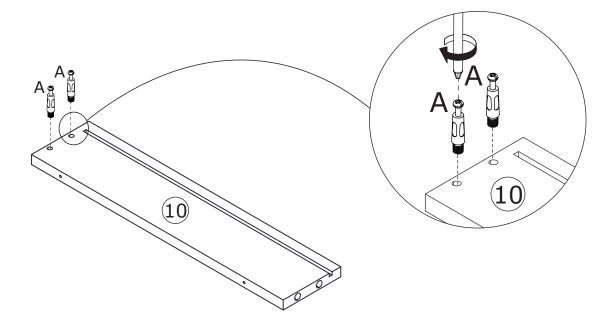
Insert quickfit screw(A) into plate 10 and 11 with a screwdriver as shown.
