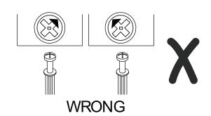
Nut should be in the centred of the cam lock when the two panels are joined.
