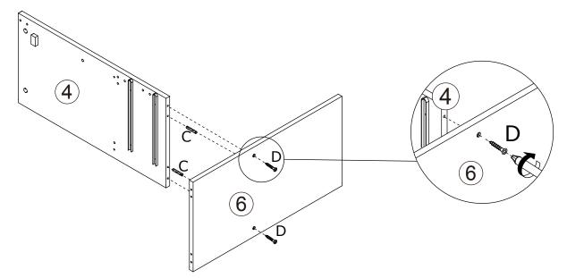
Using screw(D) to connect panel #6 with panel #4 as shown.
