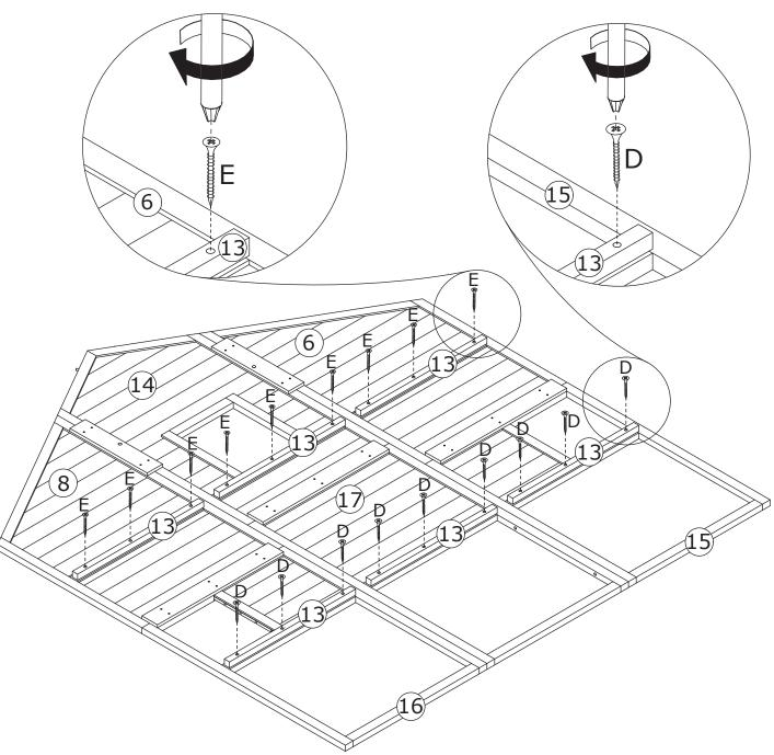
Fix plate 13 to plate 6, 8 and 14 with screw(E) as shown. Fix plate 13 to plate 15, 16 and 17 with screw(D) as shown.
