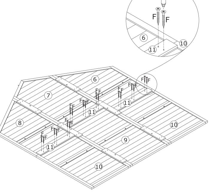
Fix plate 11 to plate 8 and 10 with screw(F) as shown. Fix plate 11 to plate 7 and 9 with screw(F) as shown. Fix plate 11 to plate 6 and 10 with screw(F) as shown.
