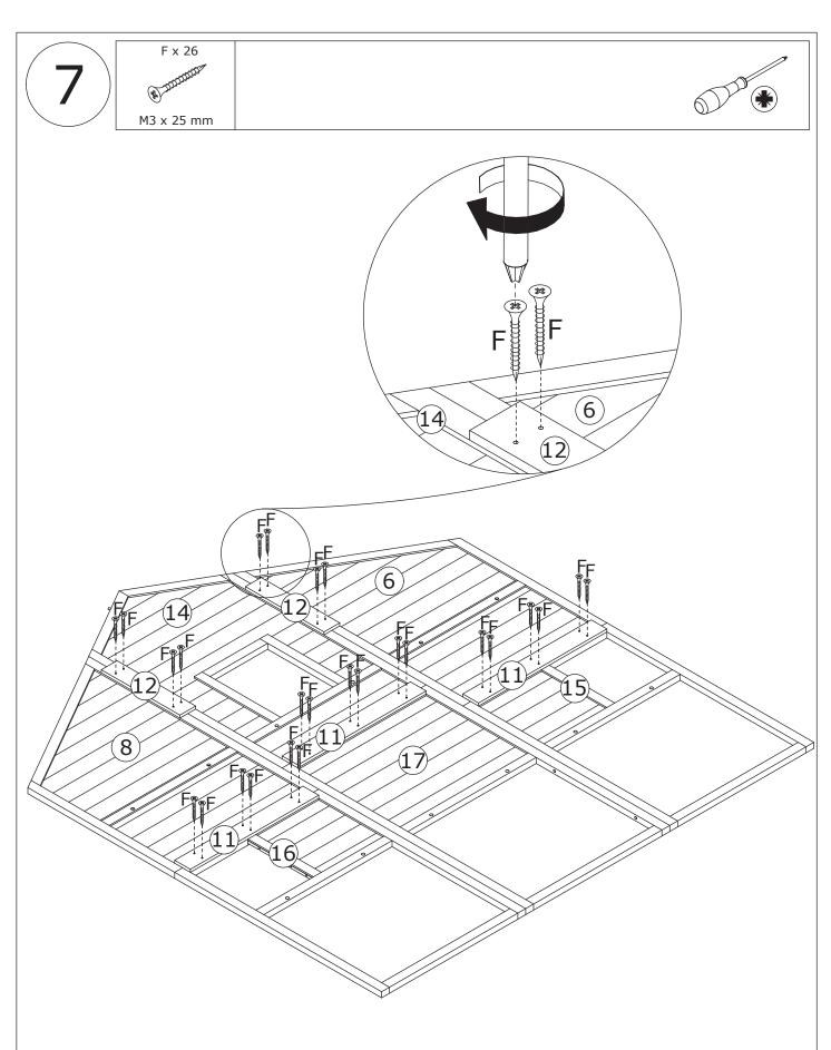
Fix plate 12 to plate 8, 6 and 14 with screw(F) as shown. Fix plate 11 to plate 6, 15, 14, 17, 8 and 16 with screw(F) as shown.
