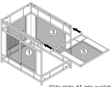
Slide plate #5 into available slots of the component(assembled in step 2) as shown.
