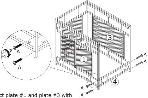
Connect plate #1 and plate #3 with plate #4 using screw(A) as shown.
