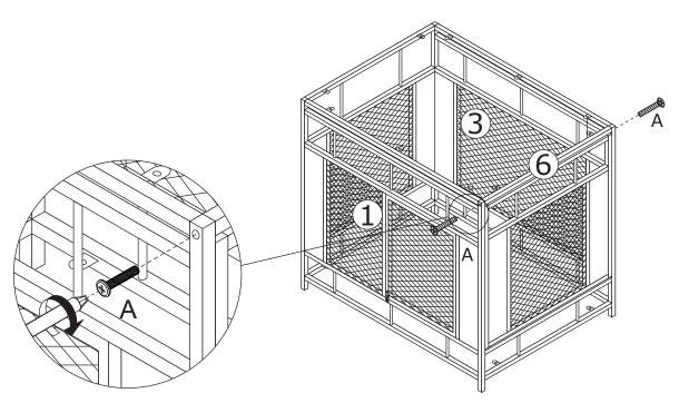
Connect plate #1 and plate #3 with plate #6 using screw(A) as shown.
