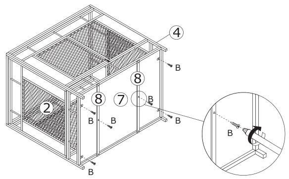
Fix plate #7 to the bottom of component (assembled in step 5) using screw(B) as shown.
