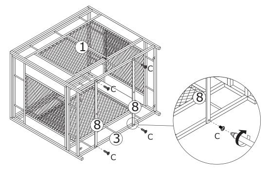
Fix plate #8 to the bottom of component (assembled in step 4) using screw(C) as shown.
