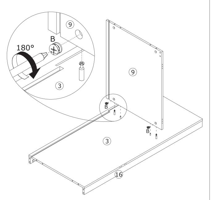
Attach board 9 to board 3, add cam lock(B) into board 9 and turn clockwise to tighten as shown.
