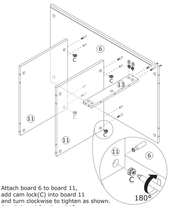
and turn clockwise to tighten as shown. Attach board 6 to board 13, add cam lock(B) into board 13 and turn clockwise to tighten as shown.
