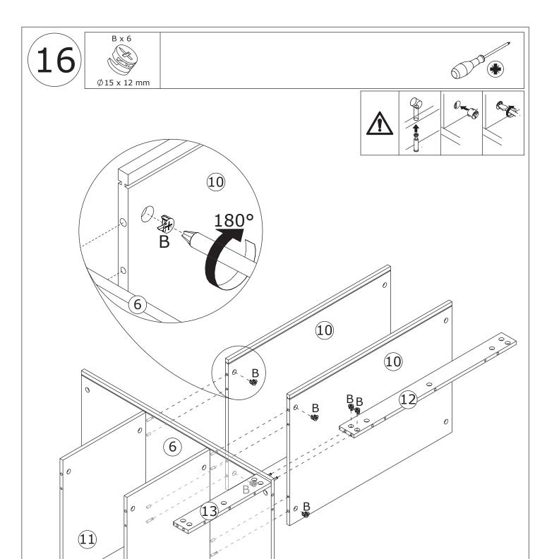
Attach board 10 and 12 to board 6, add cam lock(B) into board 10,12 and turn clockwise to tighten as shown.
