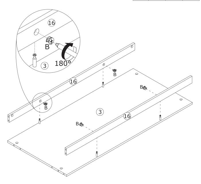
Attach board 16 to board 3, add cam lock(B) into board 16 and turn clockwise to tighten as shown.
