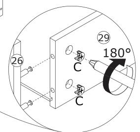
Attach board 26 to board 28 and 29, add cam lock(C) and turn clockwise to tighten as shown.
