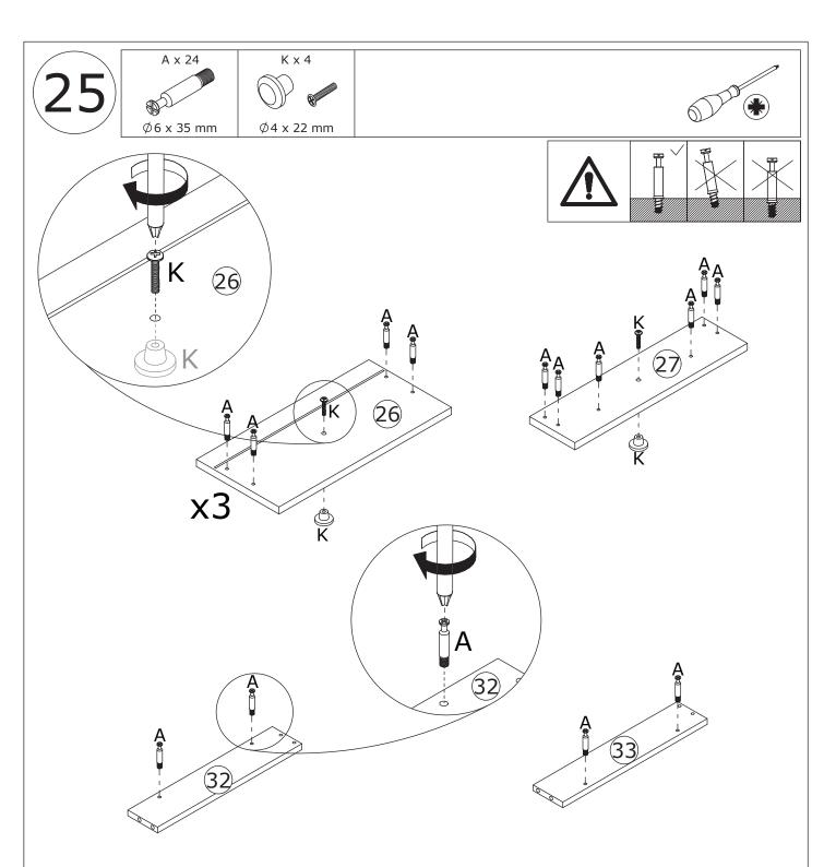
Screw eccentric rod(A) into board 26, 27, 32, 33 and 34 as shown. Fix knob(K) to board 26 and 27 as shown.
