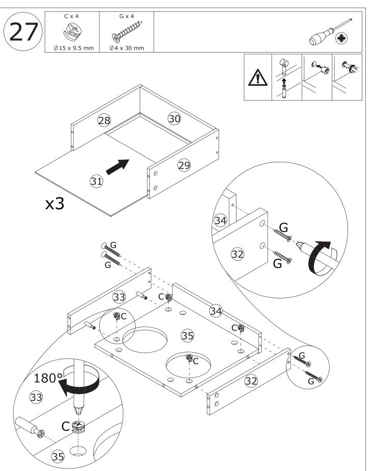
Insert bottom board 31 along grooves as shown. Attach board 33 and 32 to board 34 and 35, add cam lock(C) and turn clockwise to tighten, and fix to board 34 with screw(G) as shown.
