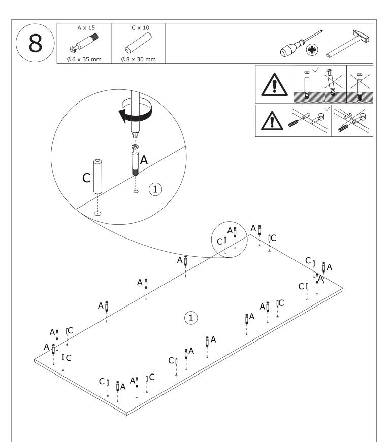
Screw eccentric rod(A) and insert wooden dowel(C) into board 1.
