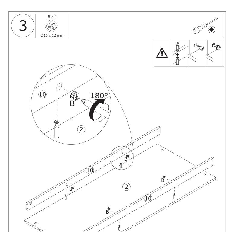
Attach board 10 to board 2, add cam lock(B) into board 10 and turn clockwise to tighten as shown.
