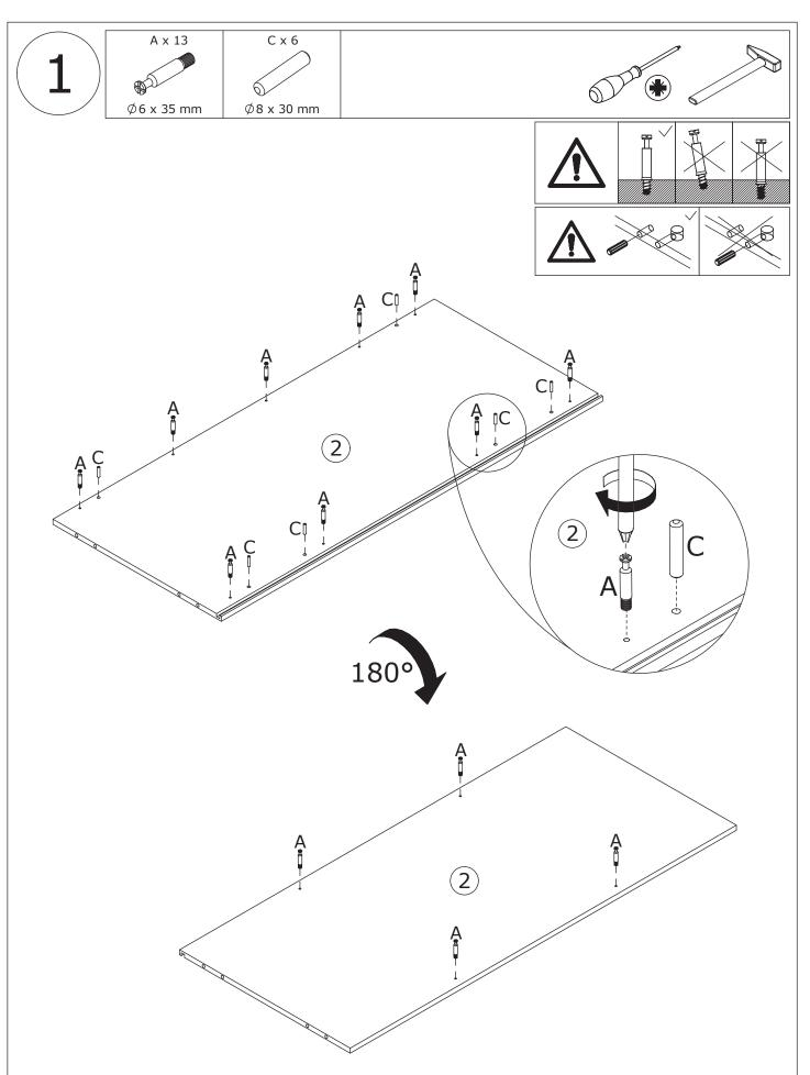
Screw eccentric rod(A) and insert wooden dowel(C) into board 2 at first. Flip the board to back, screw eccentric rod(A) into as shown.
