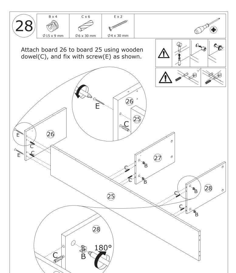
Attach board 27 and 28 to board 25 using wooden dowel(C), add cam lock(B) into board 27,28 and turn clockwise to tighten as shown.
