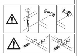
Coonnect the three assembled components using wooden dowel(C), add cam lock(B) into and turn clockwise to tighten as shown.
