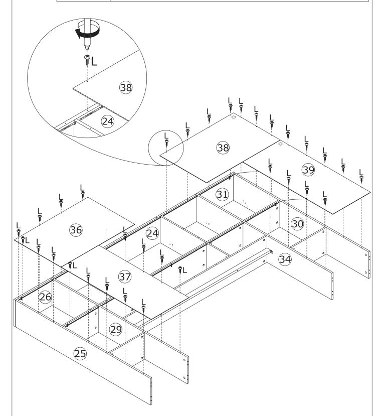
Fix back board 36, 37, 38 and 39 to the unit with screw(L) as shown.
