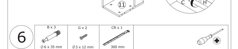
Screw eccentric rod(B) into board 3 and 10 as shown.
